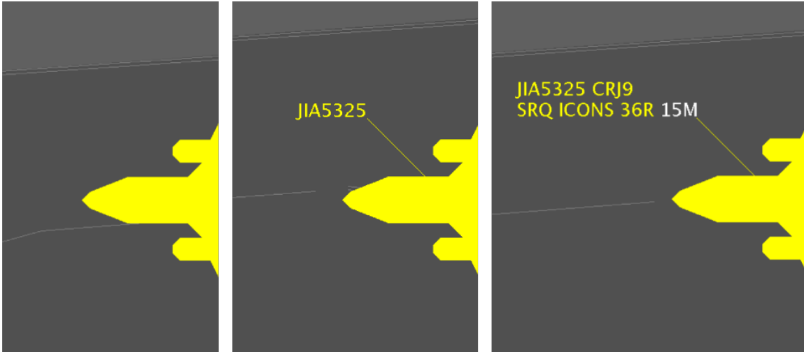
Figure 4.45. Flight Datablock Display: No Datablock (left), ID Only Datablock (middle), Extended Datablock (right).
