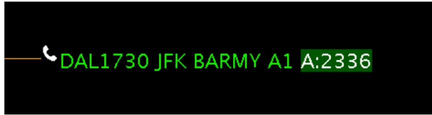
Figure 7.28. After being manually entered by the Tower, the APREQ release time is displayed in the Timeline datablock (e.g., “A:2336”).
