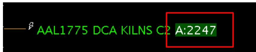
Figure 7.2. Timeline Datablock: After being scheduled, the release time (e.g., “A:2247”) is displayed.
