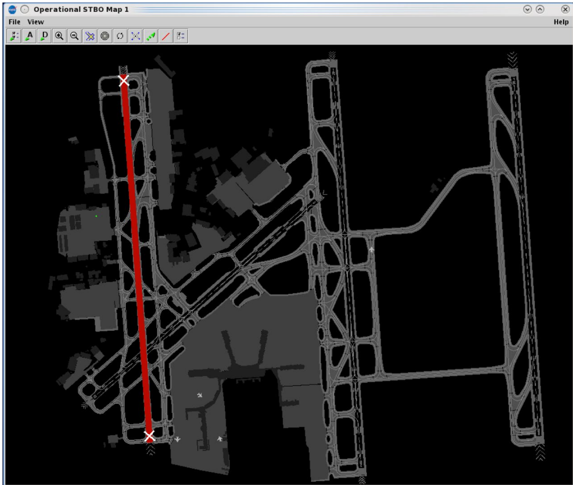
Figure 4.78. Closed runways are displayed in red with a white “X” at each end.
