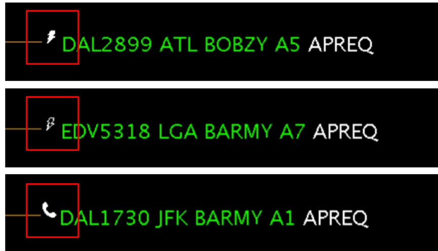
Figure 7.9. Timeline symbology indicates which TBFM/IDAC Approval Mode is being used by Center: Automatic ( solid lightning bolt ), Semi-Automatic ( hollow lightning bolt ), or Call for Release ( telephone handset ).
