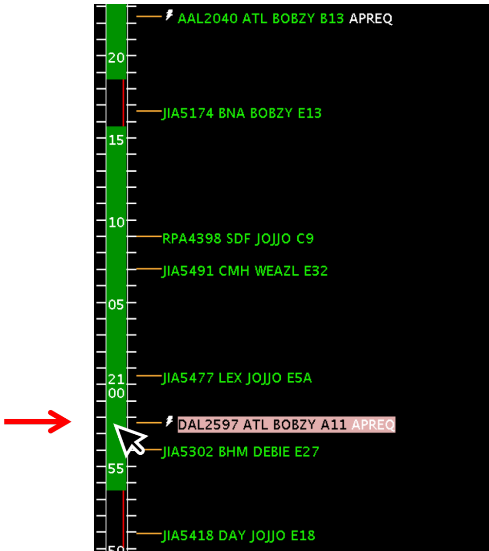
Figure 7.14. Select Slot on Timeline: Use the mouse to point and click along the timeline at the flight's predicted takeoff time.
