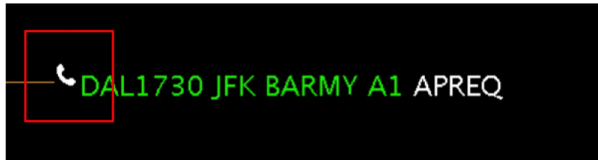
Figure 7.25. Telephone handset symbol: APREQ release time for this flight must be scheduled via Call for Release and entered manually.
