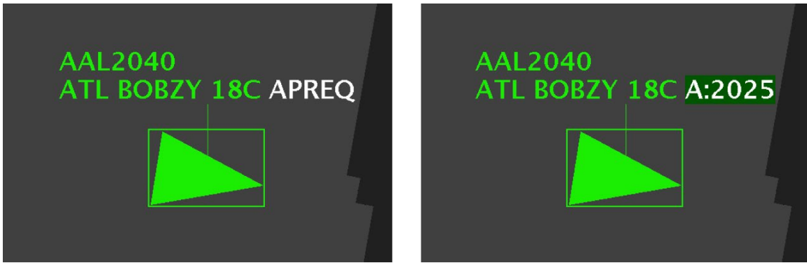
Figure 7.5. Map Datablock: Prior to being scheduled, the word “APREQ” is displayed (left). After being scheduled, the release time (e.g., “A:2025”) is displayed (right).
