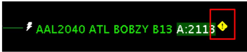
Figure 7.29. If Center changes an APREQ release time, a yellow diamond with an exclamation point is displayed in the Timeline datablock.
